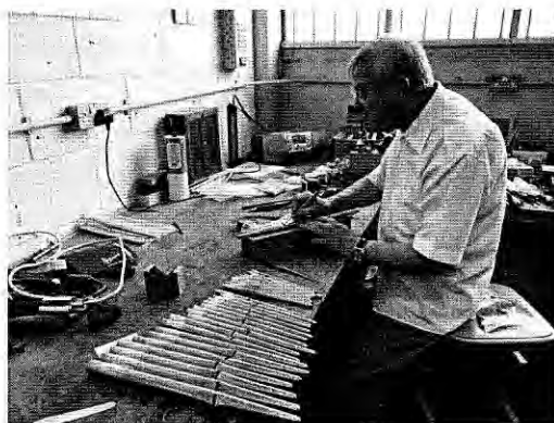
David preparing pipework for voicing
