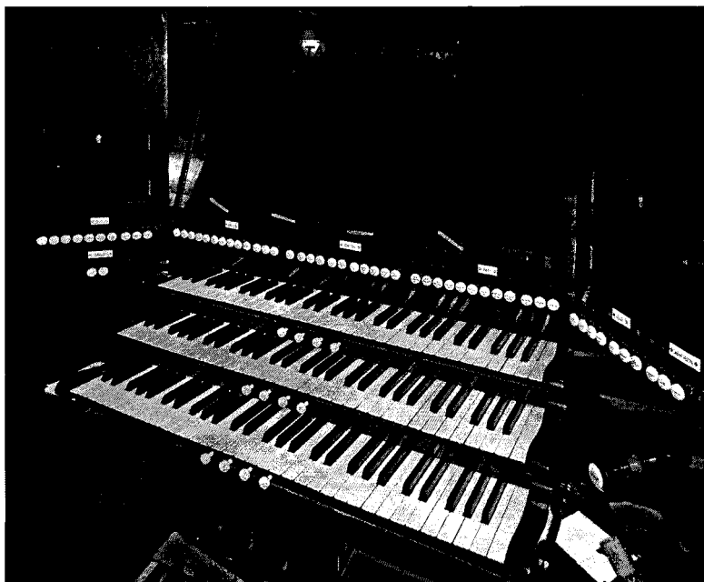
The De Montfort Hall console with characteristically small Taylor stop-heads. The single traditional knob to the lower right controls the wind. (Photo: John Norman)
