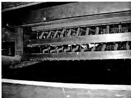
Fig. 2. Earle Rd, St Dunstan's, Edge Hill. Swell 2nd pull blow-down purses. (Photo: David Wells Organ Builders Ltd)
