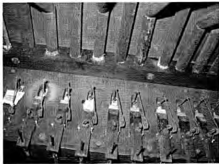
Fig. 3. Earle Rd, St Dunstan's, exhaust valves to Swell 2nd pull action. (Photo: David Wells Organ Builders Ltd)
