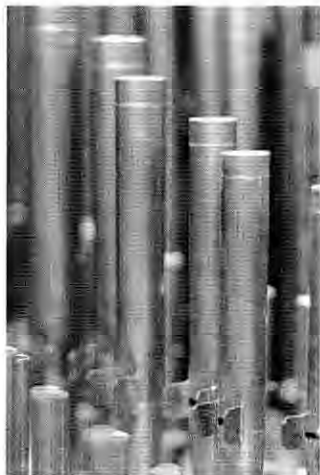
Quintadena pipes with soldered tops and tuning ears. Photo: SRB Humphreys © 2016
