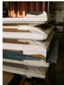
The soundboard is of pine construction, with thin cheeks, veneered with mahogany. The table and upperboards are of mahogany and the slides and bearers of oak. Seven basses of the Open Diapason and fifteen(?) of the Stopped Diapason pipes are conveyed to off-note blocks, between there of the case and the soundboard. Three crude slots have been cut in the rear panels to allow these
